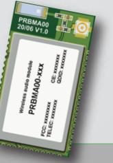
Dimension: 17 x 30 x 3mm Antenna: chip antenna, optional I-PEX connector
